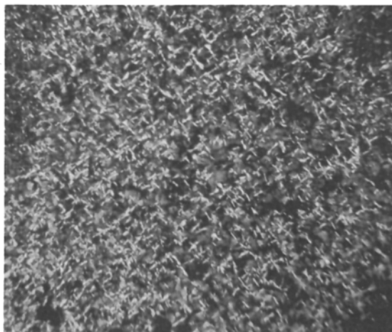
Fig. 2: Photomicrograph shows batonnet and mosaic textures. Magnification 100x, crossed polarisers.
